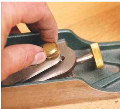
▲ A stud projection on the Norris adjuster connects to the lever cap
